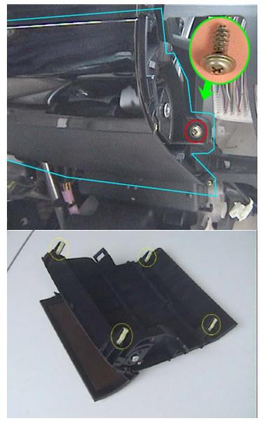
Unfortunately, you must remove the LCD touch screen before you can remove the stereo. You need a 10mm socket wrench to remove the screw circled in red and the identical one on the other side (not shown). The screws are inset, so you need a socket tool, not something like an adjustable crescent wrench. The screws may have washers behind them, so be careful not to let them fall off.
