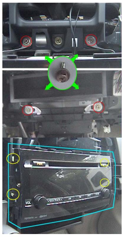
Most stereo accessories require a Y cable adapter (part #08695-00370) shown in the top two pictures to the right. The lower right picture shows this cable plugged in to the CD changer port behind the stereo (blue circle). Notice that the plug needs to be pushed much deeper than the plug next to it, which can take a significant amount of force (try pushing with the wide tips of a pliers).
