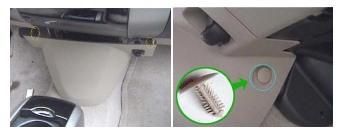
Once you get the fastener pulled out, the panel is held on by two neon-yellow snaps circled in yellow in the left picture, above. To get the snaps out, you can get one hand behind each side of the panel and just pull it firmly.
