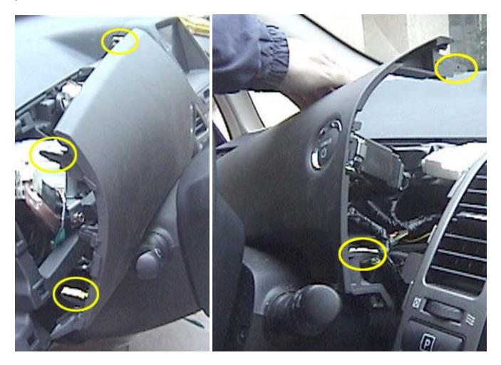
Now, you can finally remove the silver vent to the left of the stereo (outlined in blue in the upper picture to the right). It is held on by 5 snaps (circled in yellow). This panel is much easier to remove than the other vents because you can get your fingers behind it on the left. The shift knob is not attached to this panel and will slip out through a circular hole.
