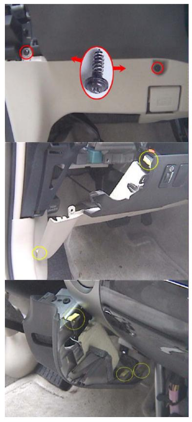
Next, remove the panel above the steering wheel. It is held on by four yellow snaps (two on the right and two on the left). It should be easy to get behind it with your fingers. Once popped off, a wire from the start button will prevent you from pulling the panel too far back, so just let it hang.
