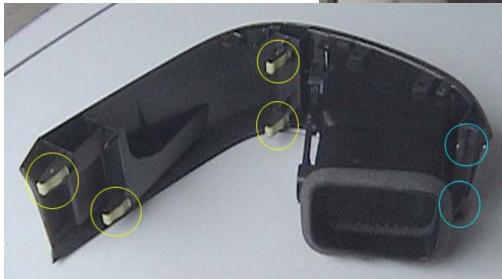
Next, you can remove the tan plastic piece below the stereo, shown snapped out in the picture below.
