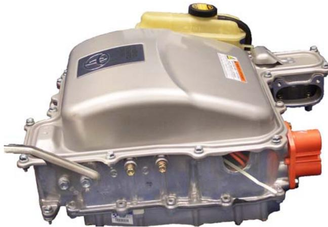
**Fig. 2.9. 2004 Prius inverter and voltage converter unit.**
